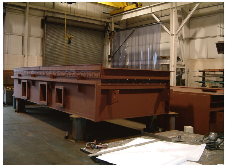
Assembled Stoker, blocked for inspection.
