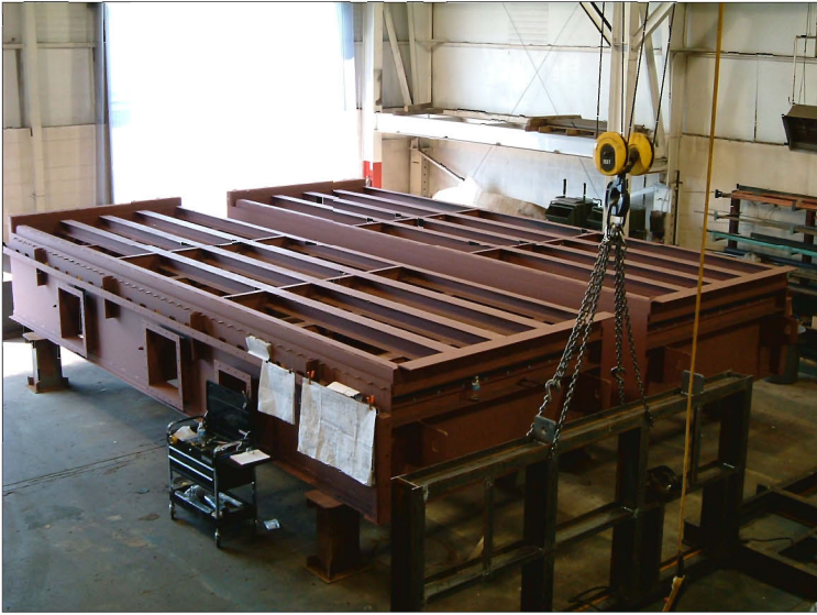
Fixed Frame with vibrating frame installed - No Grates.
