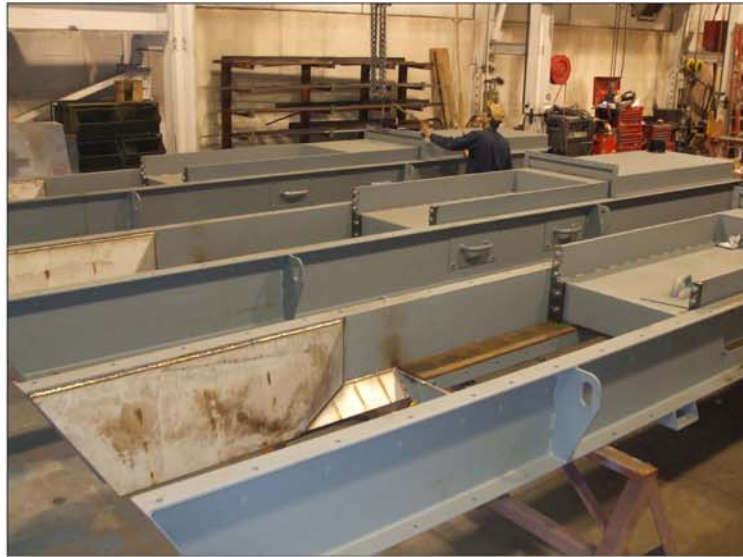
RDF Feed Ram during assembly.
