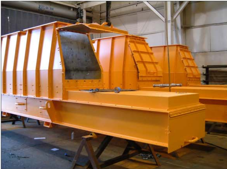
Final assembly of the RDF Feed Ram near completion Door latches, gasketing and signage to be added. Three (3) Rams required for job.
