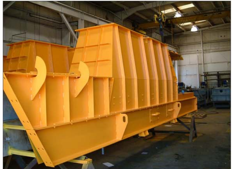
Final assembly of the RDF Feed Ram near completion Door latches, gasketing and signage to be added. Three (3) Rams required for job.
