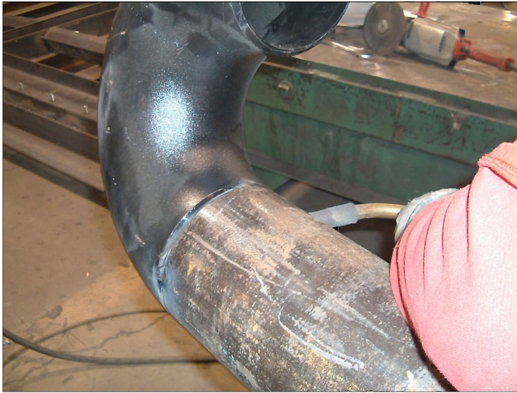
Burner tube welding.
