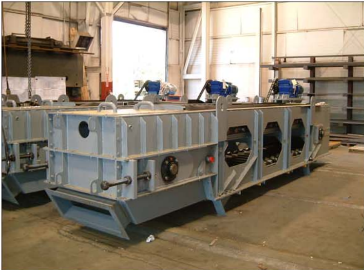
Conveyor Assembly near completion. A total of three (3) conveyors are required for job.
