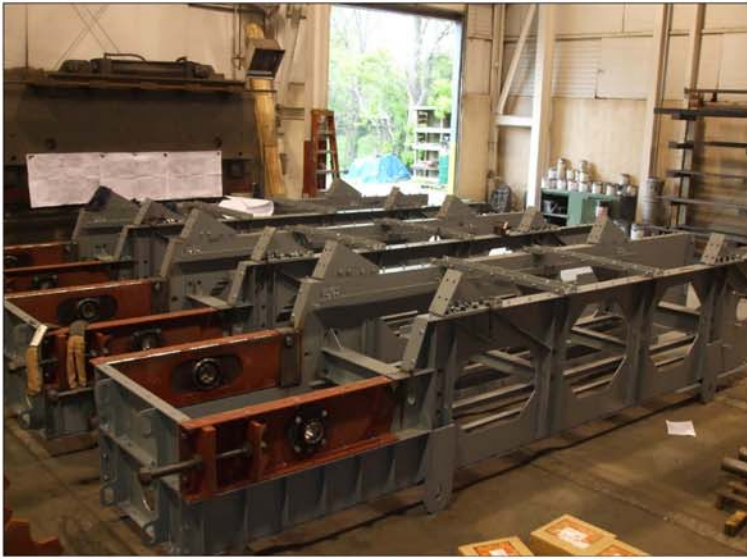
Begin Apron Chain Conveyor Assembly
