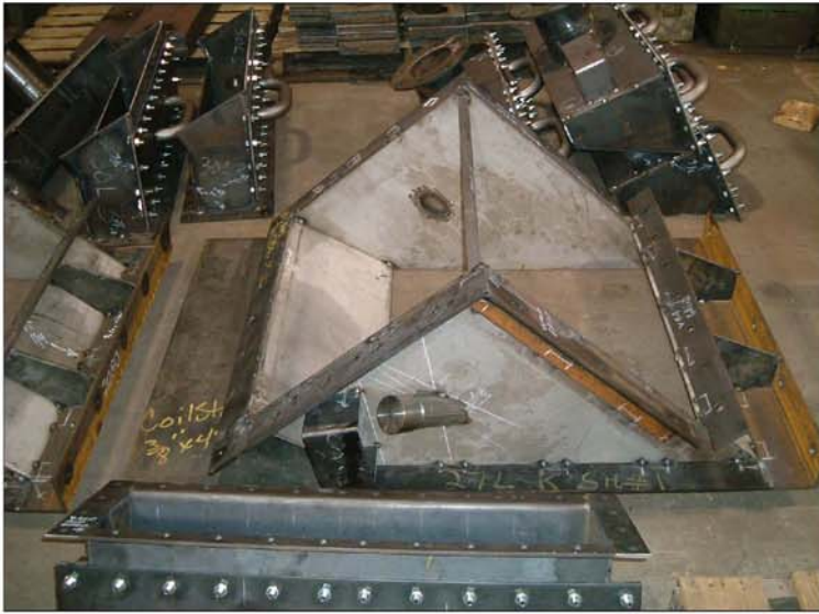
Chute fit-up prior to final welding.
